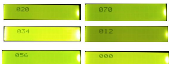
Fig 5.4 LCD Displayed Output of 4-tap WP FIR Filter using DA
