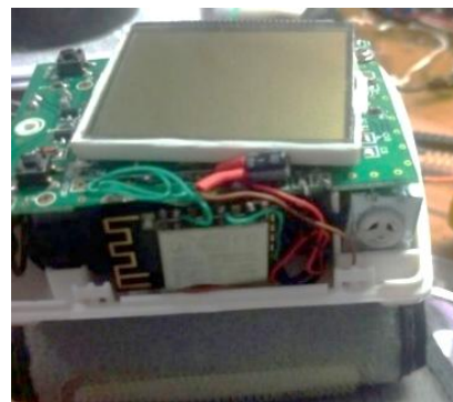
Fig.5. ESP8266 module embedded in a digital A Digital Tension meter device
