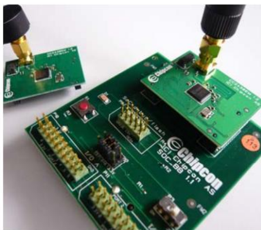
Figure 4. Zigbee modules used in this project. On the left is a stand alone Zigbee module, to the right is a module installed on the development board.
