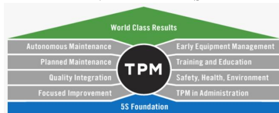
Figure 2: The traditional TPM model consists of a 5S foundation and eight supporting activities
