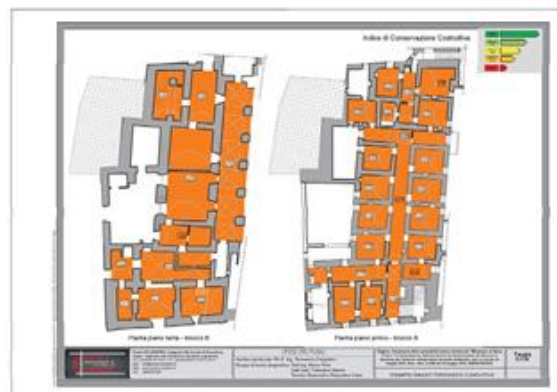
Figure 6: Constructive conservation Assessment of masonry horizontal bearing solutions macroblock B.
