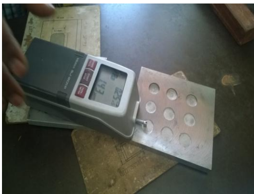
Fig.2.3 Measuring of surface roughness by using taly surf meter.
