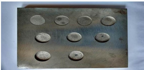
Fig.2.2 Work pieces after machining with waste palm oil blended with kerosene and kerosene as dielectric fluids.
