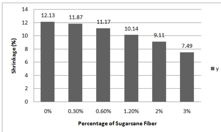
**Fig.4.** Shrinkage percentage by sugarcane fiber mix.
