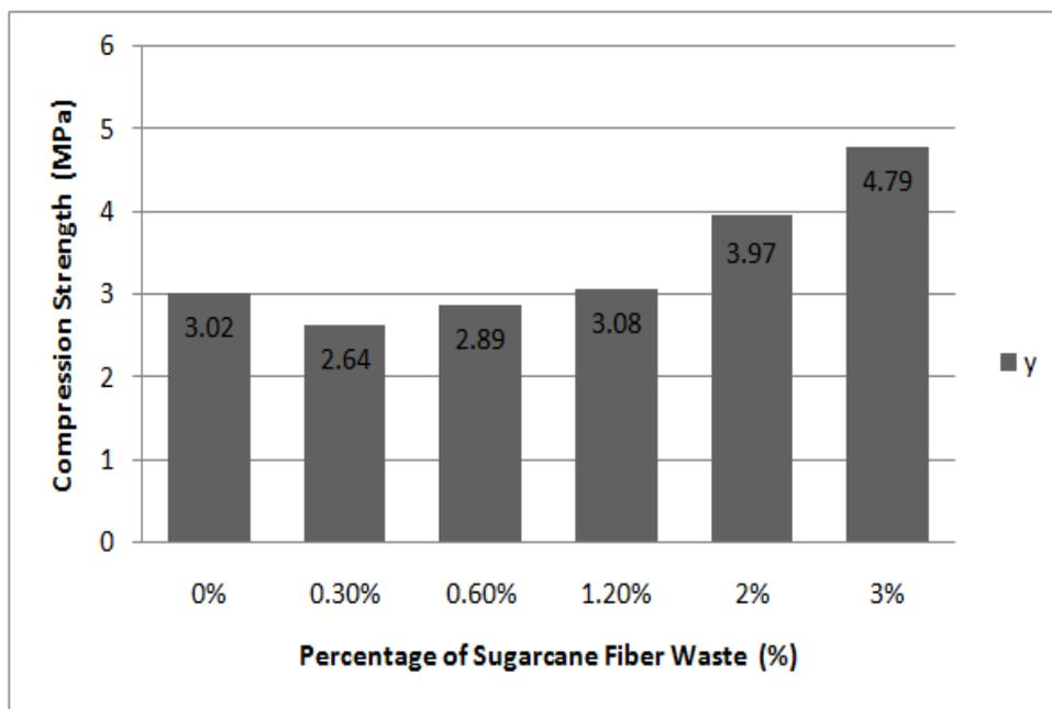
**Fig.5.** Compression strength by percentage of sugarcane fiber waste
