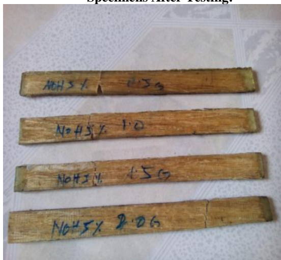
Fig. Without NaOH treatment of banana fiber polyester composites after tensile testing
