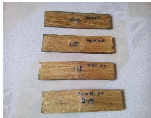
Fig: NaOH treatment of banana fiber polyester composites after bending test.
