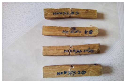
Fig: NaOH treatment of banana fiber polyester composites after impact test.
