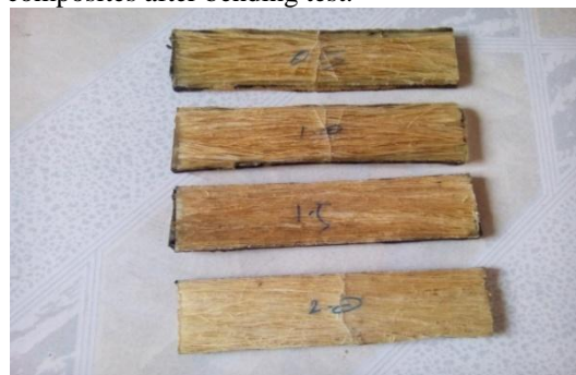
Fig: Without NaOH treatment of banana fiber polyester composites after bending test.
