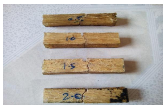
Fig: Without NaOH treatment of banana fiber
