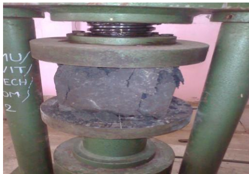
Figure 1 Compressive Strength test on Sandcrete Blocks
