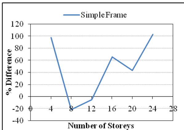
Fig. 14: Percentage Difference of Steel Weight Between Conventional and Diagrid Systems
