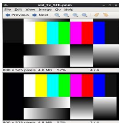
c) A Frame Colour Bar of 640x480p Format Figure 3 HDMI Transmitter Model Video Verification
