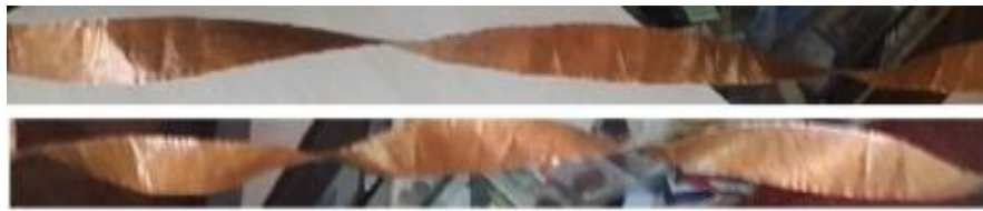
Figure no: 2. the inner tube fitted with twisted tape at different twist ratios ( \gamma = 7.0 and 5.0 )
