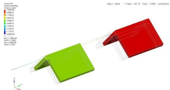
Figure 7. Result of modal analysis: 1st mode of vibration in 2.789Hz
