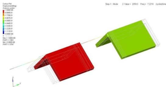
Figure 8. Result of modal analysis: 2nd mode of vibration in 7.222Hz
