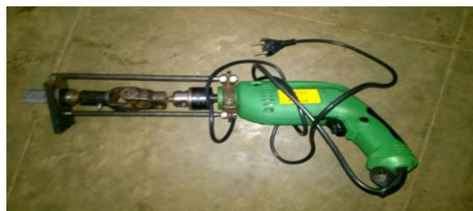
Figure 5. Top view of square hole drilling machine
