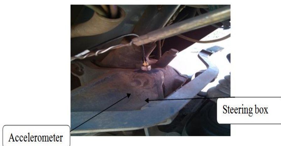
Fig: Accelerometer mounting at steering box
