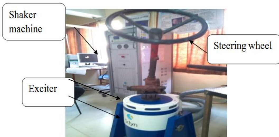
Fig: steering system is mounted on shaker machine
