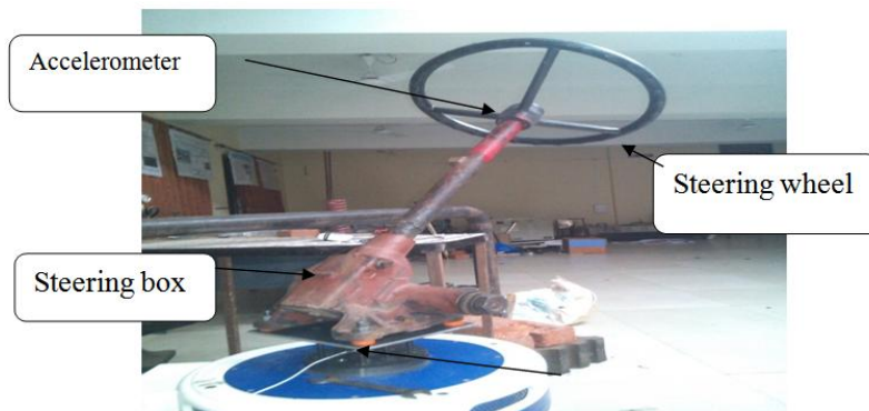
Fig: Experimental setup on shaker with damper
