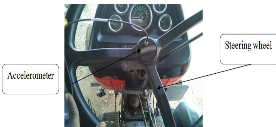
Fig: Accelerometer mounting on steering wheel (running)
