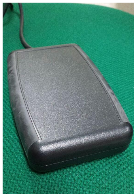
Fig 1. Multi ISO Reader (OK 5553) RFID for reading and writing on cards and tags.
