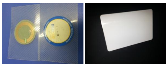
Fig 2. Mifare (ISO 14443) and RFID (ISO 15693) tags for recording personal data of owners (guest).
