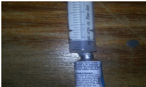
Plate 2. Sucking of healing agent into syringe
