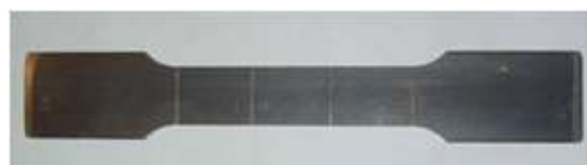
Figure 11a: Specimen for the tensile tests
