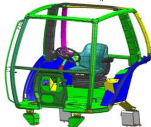
Figure 3: Structural part of the cabin
