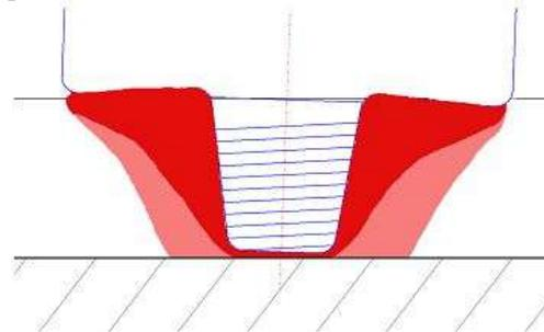
Fig. 5 drawing showing the plunge depth and tilt of the tool [1]
