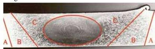
Fig. 2. Micro structural zone classification in a friction stir weld in Al 2024 alloy (A: parent material, unaffected by process; B: HAZ, thermally affected but with no visible plastic deformation; C: TMAZ, affected by heat and plastic deformation) [1]
