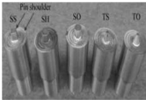
Fig.4. Image of manufacture tool with different tool profile [15]
