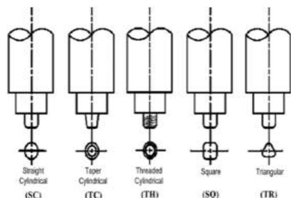
Fig.3. Types of tool pin profiles [14].
