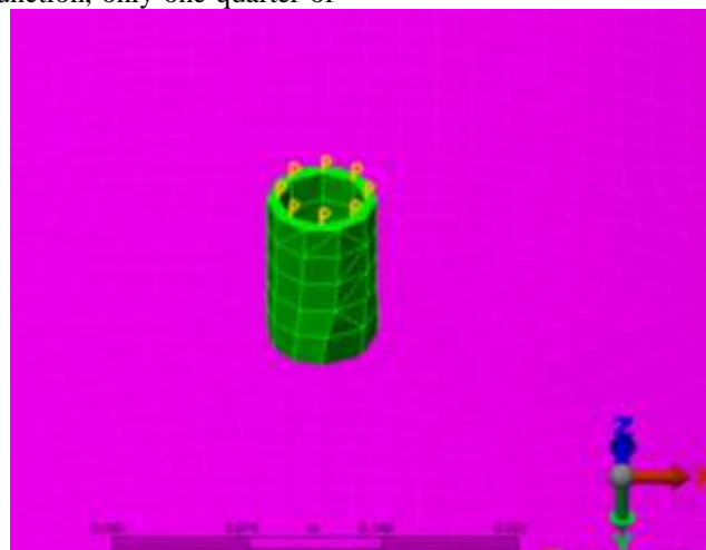
Figure 5 - Perspective view of junction nozzle/vessel – Nozzle 2”
