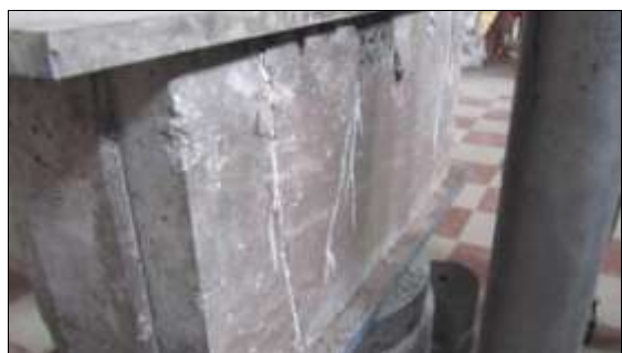
Fig 14. Failure Pattern of CHB
