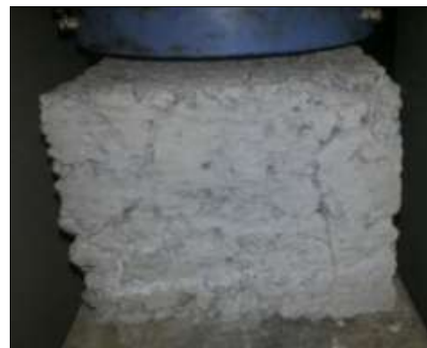
Fig 12. Failure Pattern of SB
