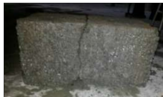
Fig 13. Failure Pattern of HB
