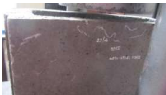
Fig 14. Failure Pattern of CHB
