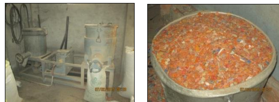
Fig 2 Shredding and Shredded HDPE Materials
