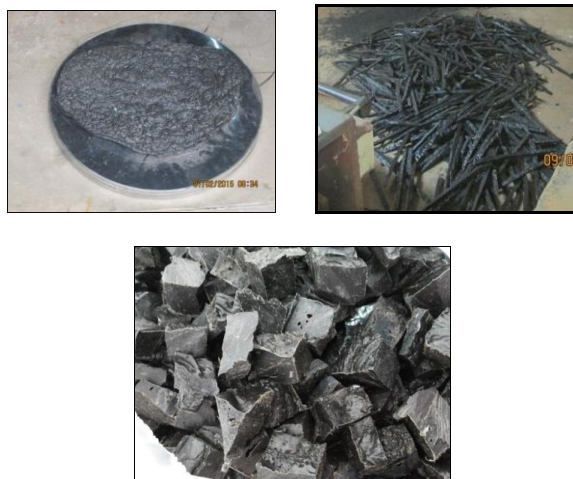
Fig 5 Making and Cutting of Plastic Sheets into Aggregate
