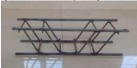
**Fig.1 Reinforcement of Beam RSB**
