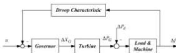
Fig. 2.1.Linear model of a single-area power system. performance of load frequency control system, i.e.,  $u = -K(s)\Delta f$  find a control law , where K(s) takes the form
