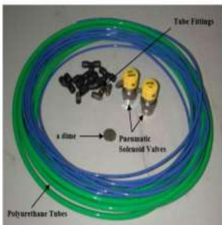
Figure 3-7 Polyurethane Tubes, Tube Fittings, and Pneumatic Solenoid Valves
