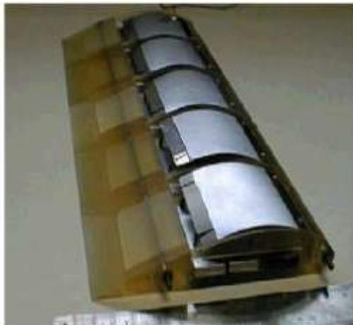
Figure 2-20 Wing Plan-form With Separate Controlled Actuator in Each Module
