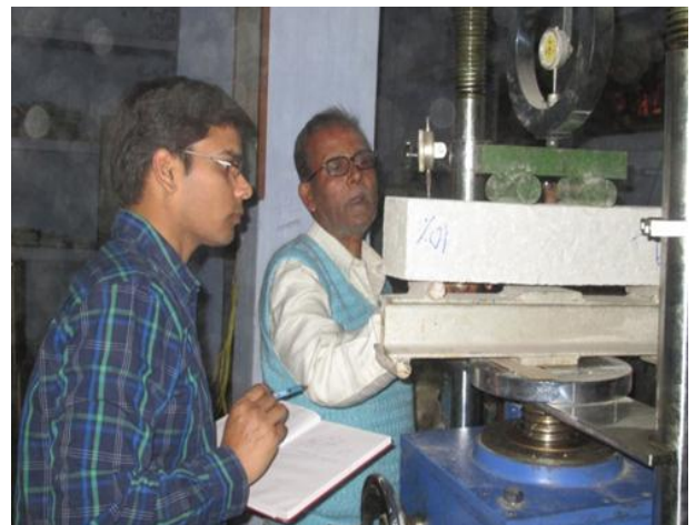
Fig. 4.4 Experimental setup for flexural testing machine
