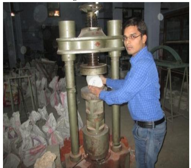
Fig. 4.4 Experimental setup for flexural testing machine
