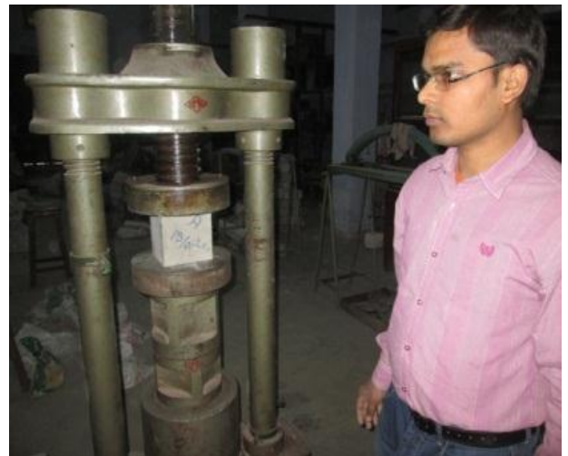
Fig.4.3 Experimental setup for split tensile strength machine.
