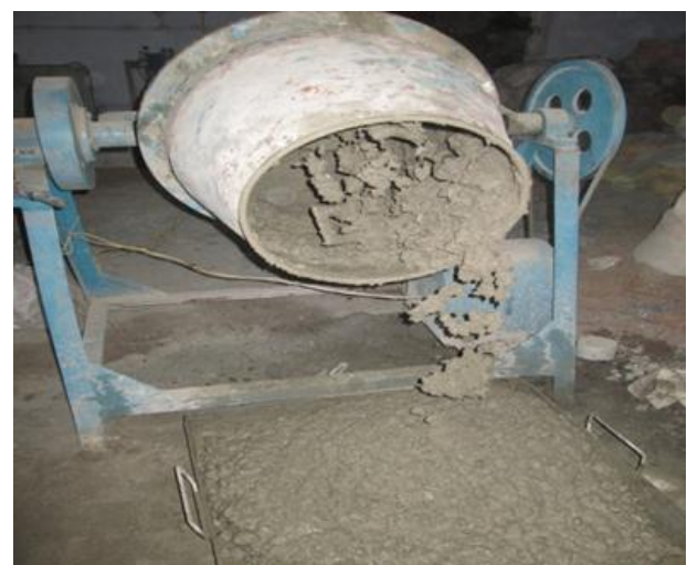
Figure4.1 Mixing Process in Standard drum type mixer
