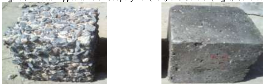
Figure 9: Visual Appearance of Geopolymer (Left) and Control (Right) Concrete
