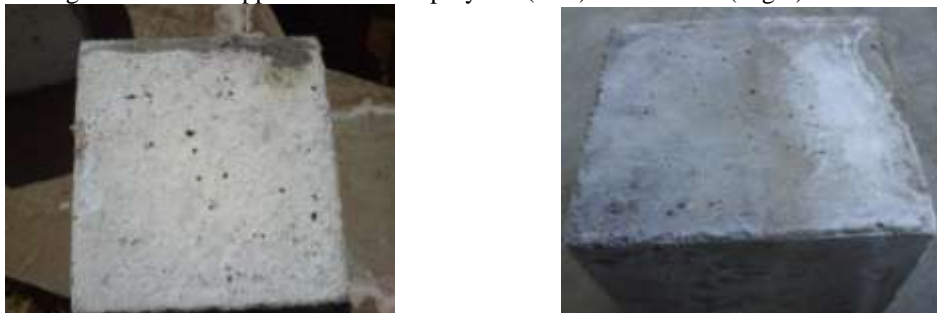
Figure 5. Visual Appearance of Geopolymer (Left) and Control (Right) Concrete
