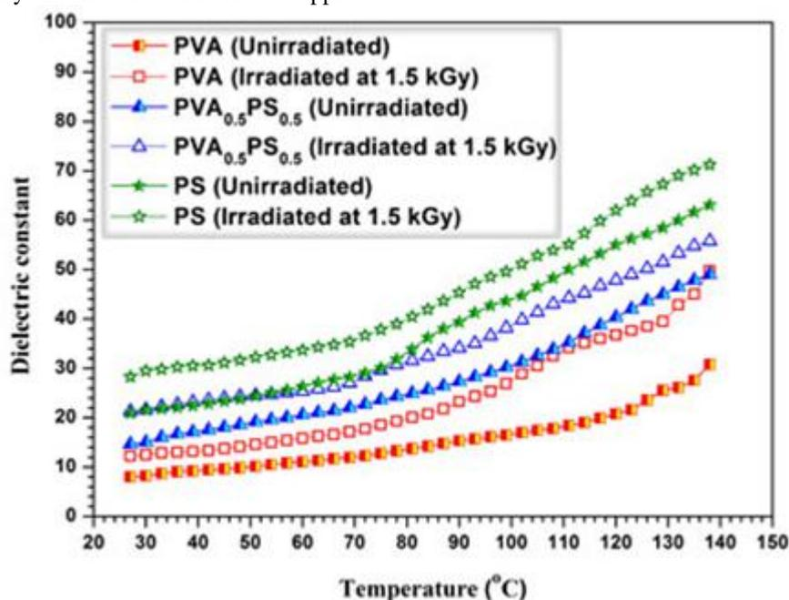
**Fig. 2:** Variation of the dielectric constants for PVA, PVA<sub>0.5</sub>PS<sub>0.5</sub> and PS films as a function of temperature at constant 1 kHz frequency.
