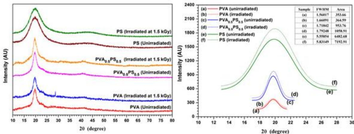
Fig. 1: (a) X-ray diffraction patterns of unirradiated and irradiated PVA, PVA<sub>0.5</sub>PS<sub>0.5</sub> and PS films (b) Gaussian function fitted curves for high intensity broad peak
