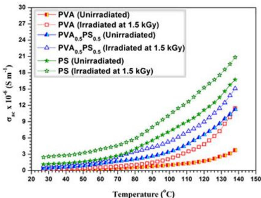
Fig. 4: Variation of the AC conductivity ( $\sigma_{ac}$ ) for PVA, PVA<sub>0.5</sub>PS<sub>0.5</sub> and PS films as a function of temperature at constant 1 kHz frequency.
