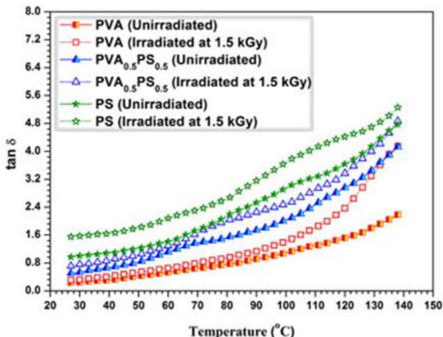
Fig. 3: Variation of the dielectric loss ( $\tan\delta$ ) for PVA, PVA<sub>0.5</sub>PS<sub>0.5</sub> and PS films as a function of temperature at constant 1 kHz frequency.
