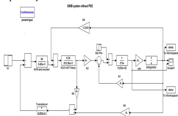
Fig. 4 Simulink diagram without PSS
