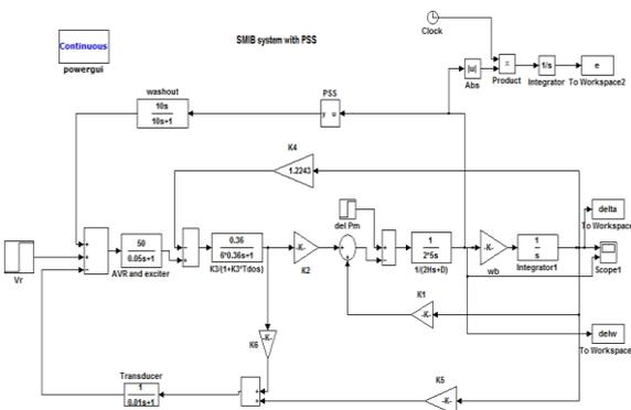
Fig. 5 Simulink diagram with PSS
