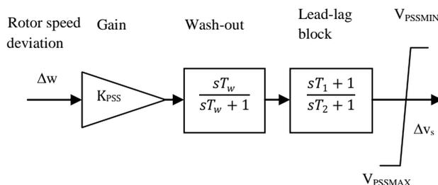
Fig. 2 Basic Power system stabilizer
