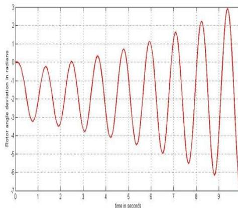
Fig. 6 Rotor angle deviation without PSS
