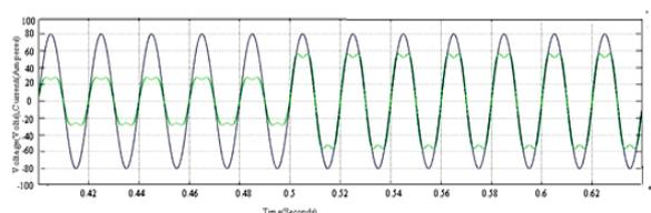
**Fig.4 (i) Compensated voltage and distorted current**
