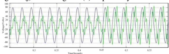
**Fig.4(h) Load Voltage with and without Compensation**
