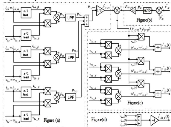
**Fig .3 (a) Calculation of Per phase Fundamental Active Power (b) DC link voltage control loop (c) The Generation of Reference source current (d) Neutral Current Compensation.**
