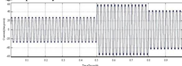
**Fig.4(f) Load current variations with changed load**
