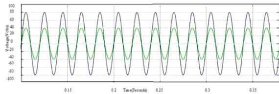
**Fig.4 (a) The Phase to neutral voltage and grid current for the phase 'a'**
