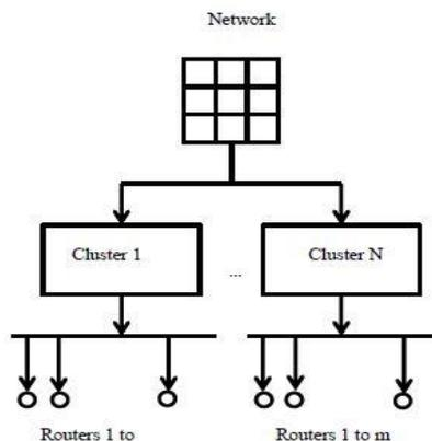
Fig2.CBHR Concept in NoC Architecture
