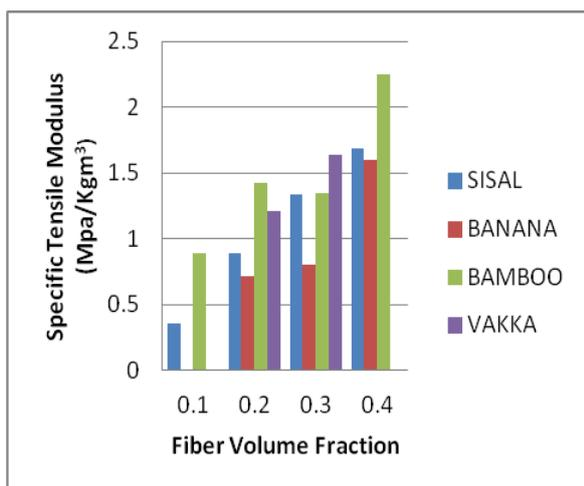
Fig.10- Volume fraction Vs specific tensile modulus of different natural fibers.
