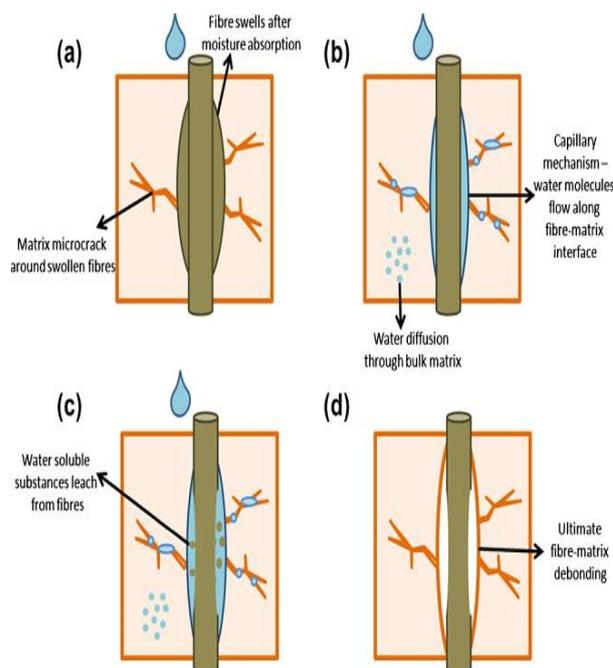
Fig.9- Effect of moisture on fiber – matrix interface [14].
