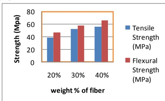
Fig.7-Effect of fiber content on tensile and flexural strength of sisal/coir epoxy composite
