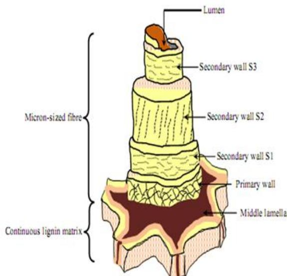
Fig.3 Typical Structure of a natural fiber. [5]
