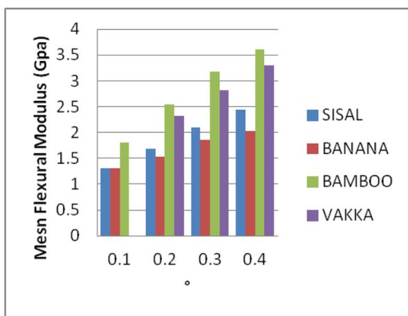
Fig.11- Volume fraction Vs and mean flexural modulus of different natural fibers.
