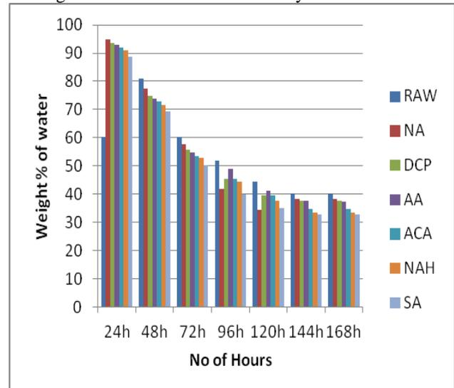
Fig.5 .comparative water retention by coir fiber subjected different surface treatment techniques.
