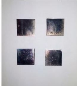
Figure 2: SS316L Plate after zirconium coating(cut into four pieces by wirecut EDM)
