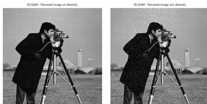
Fig. 8 Received image using 16-QAM at SNR= 10 dB with and without diversity.
