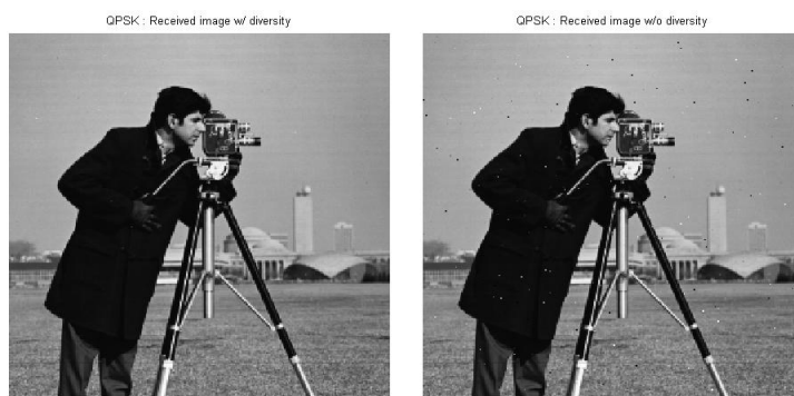
Fig. 7 Received image using QPSK at SNR=10 dB with and without diversity.
