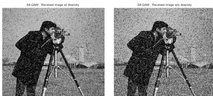
Fig. 9 Received image using 64-QAM at SNR=10 dB with and without diversity.
