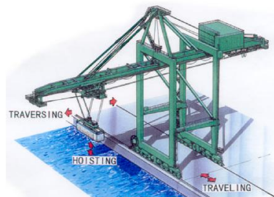
Fig.1. Container Crane Mechanism [4]
