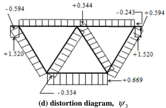
Fig. 1: Generalized strain modes for the multi-cell trapezoidal box girder section
