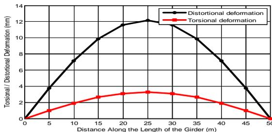
**Fig.6: Torsional and distortional deformations along the length of the girder**
