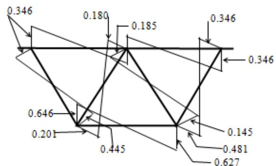
Fig.2: Distortional bending moment diagram for the multi-cell box girder
