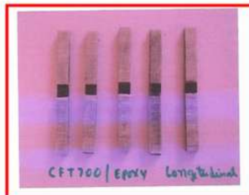
FIGURE 15: (b) The Compressive Test Results of laminate specimen's and Failure modes Of test specimen's
