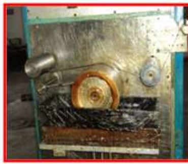
FIGURE 6: Fabrication of Carbon Fibre /Epoxy resin UD Laminate by Filament Winding Process
