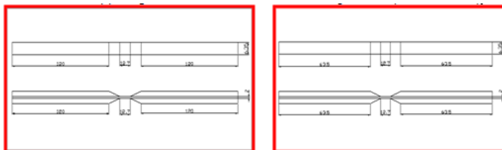
FIGURE 10: (b) Longitudinal & Transverse Compressive Test Specimens (ASTM D 3410)
