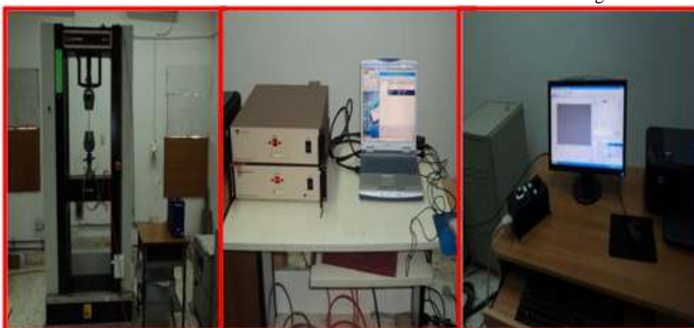
FIGURE 14: (a) The Tensile testing of UD laminate specimens in UTM with strain gauge data logger system
