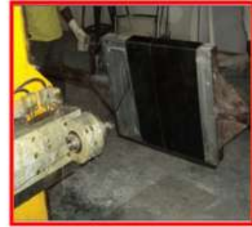
FIGURE 6: Fabrication of Carbon Fibre /Epoxy resin UD Laminate by Filament Winding Process
