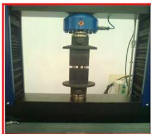
FIGURE 15: (a) The Compressive IITRI Test Fixture & Test Results of laminate specimen's
