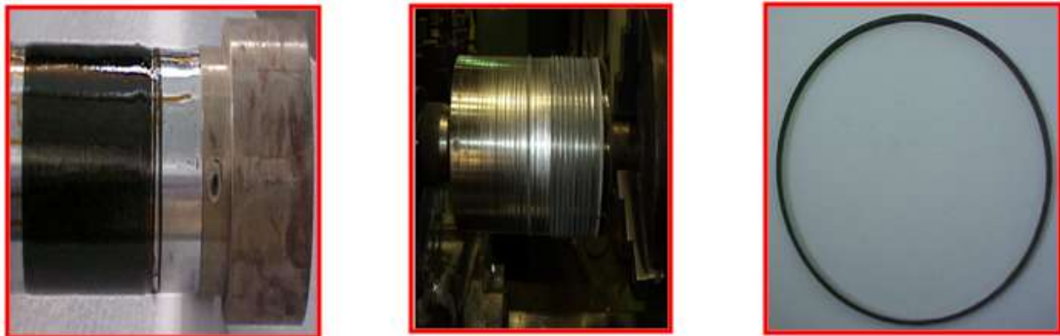
FIGURE 9: NOL winding and partition of winding into rings
