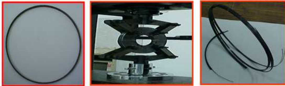
FIGURE 11: NOL Test Fixture (ASTM D 229)
