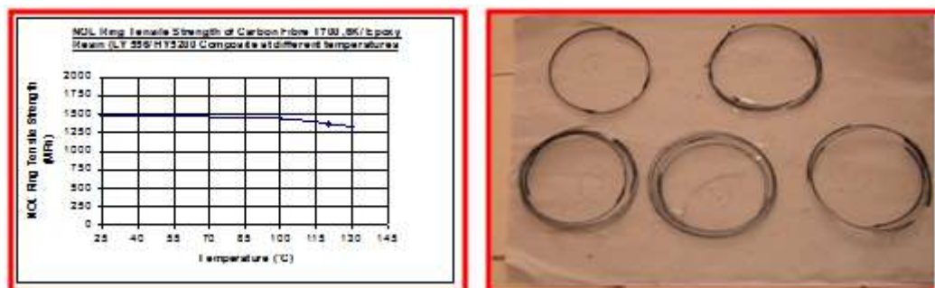
FIGURE 13: Plot for Tensile Strength Vs Temperature & NOL Rings were failed in delamination and circumferential splitting failure Test Results
