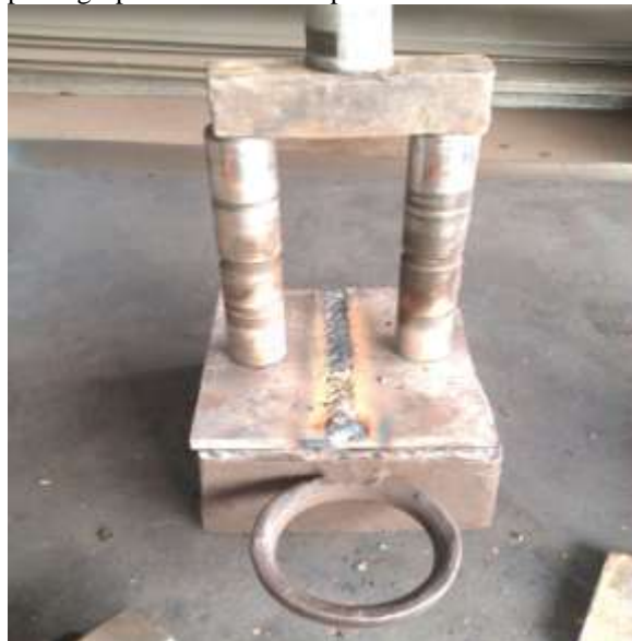
Figure 4 Welded Sample of Mild Steel
