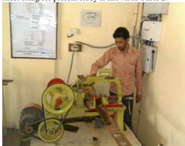
Figure 2 Cutting of Sample from Strip
