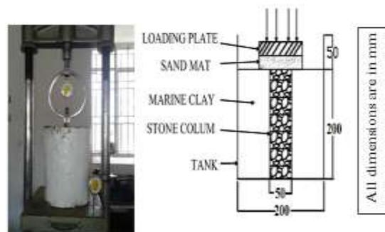
Fig: 5(a) Test setup arrangement Fig: 5(b) Schematic view of stone column
