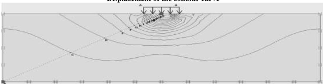
We have calculated the bearing capacity by dividing the applied load by area of the foundation. We took the height of the foundation as 1 inch and the breadth is 1 inch by convention of the 2-D software. So in every case our
