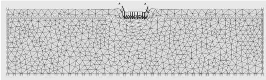
4. One geo-grid is at 0.875 inch and another one is at 0.4375 inch from the top of the foundation
