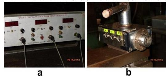
Figure 2. Electronic Dynamometer a) Digital panel b) Tool post
