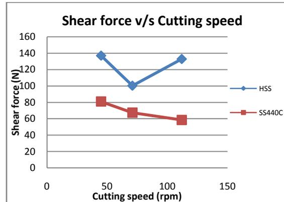
Graph 1: Shear force v/s Cutting speed
