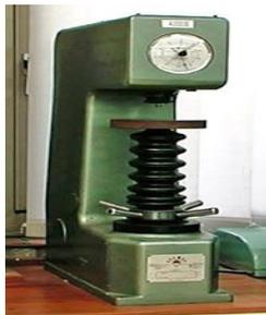
Figure 4: Rockwell hardness tester
