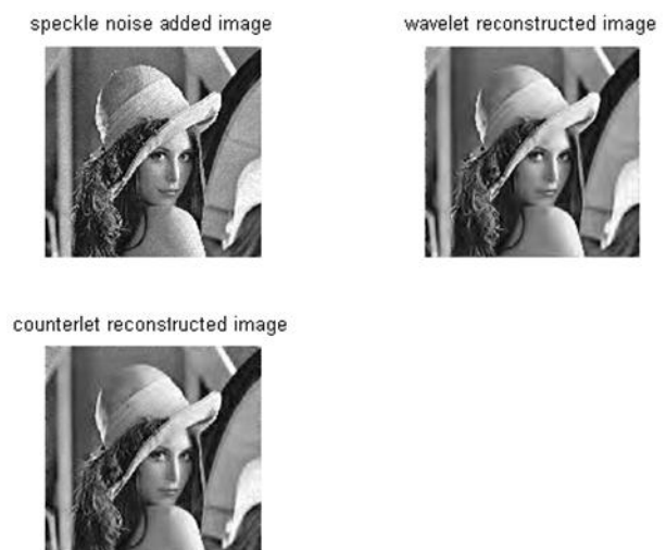
Fig. 6 Speckle noise image and denoised images using wavelet and contourlet
