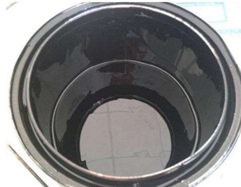
Fig2.2 asphalt of shell 90
