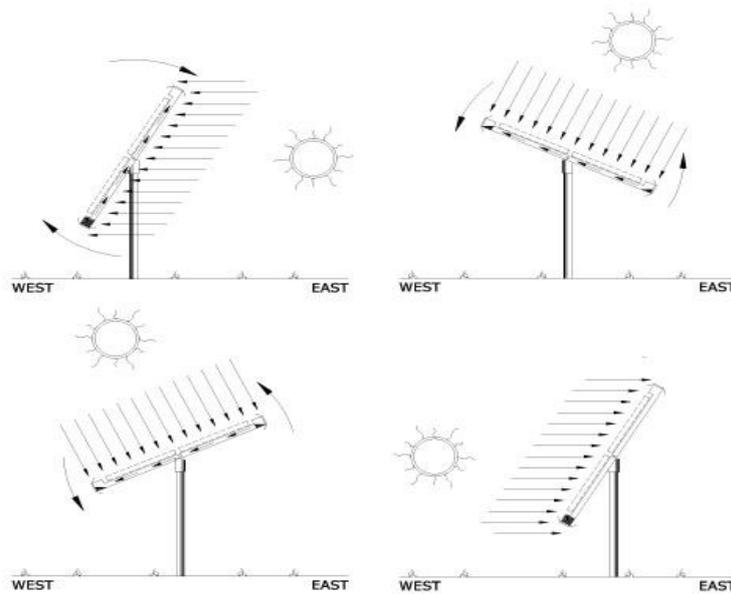
This system uses the idea of thermal expansion of materials as method for tracking. Typically a chlorofluorocarbon (CFC) or a type of shape memory alloy is placed on either side of solar panel. When the panel is perpendicular with the sun, the two sides are at equilibrium. Once the sun moves, one side is heated and causes one side to expand and the other to contract, causing the solar panel to rotate.
