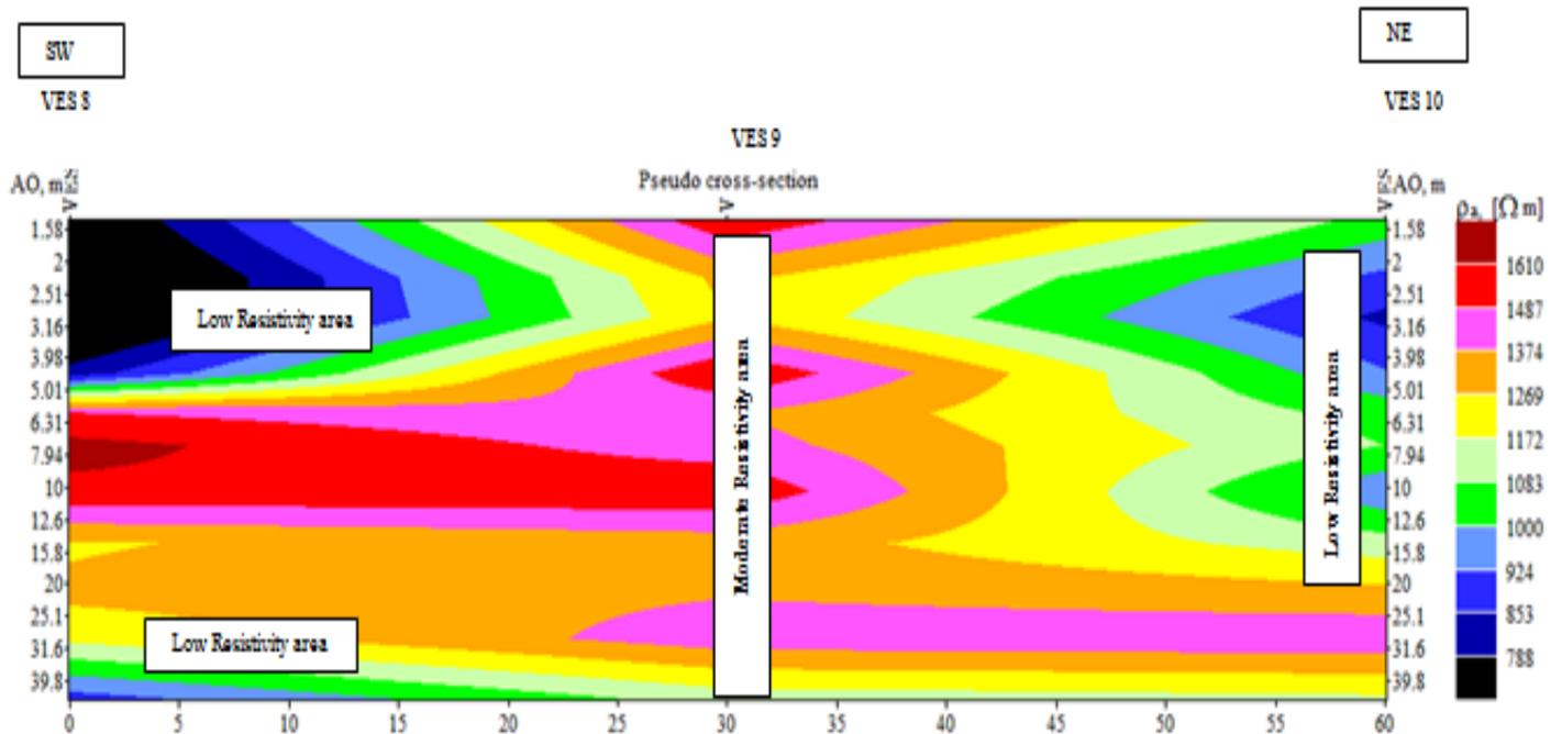
Figure 16 SW – NE Pseudo Cross Section A: (VES points 8, 9 & 10)
