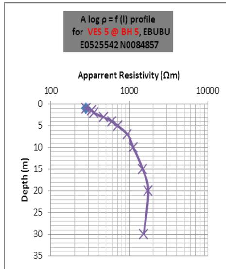
Figure 8. Resistivity log for VES 5
