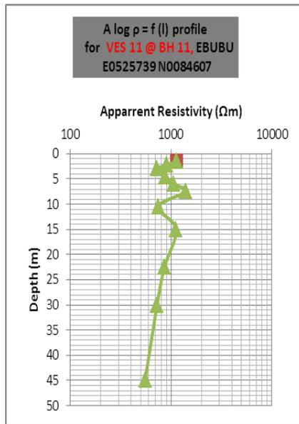
Figure 14. Resistivity log for VES 11
