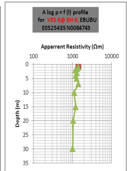
Figure 9. Resistivity log for VES 6
