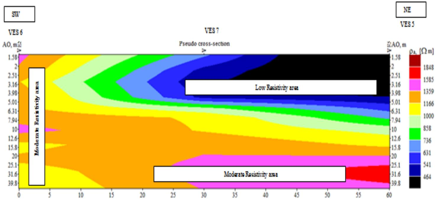
Figure 17 SW-NE Pseudo Cross Section B: (VES points 6, 7 & 5)
