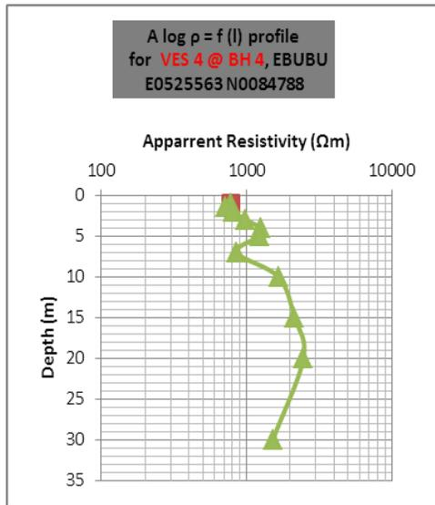
Figure 7. Resistivity log for VES 4
