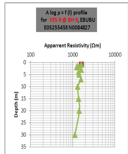
Figure 12. Resistivity log for VES 9
