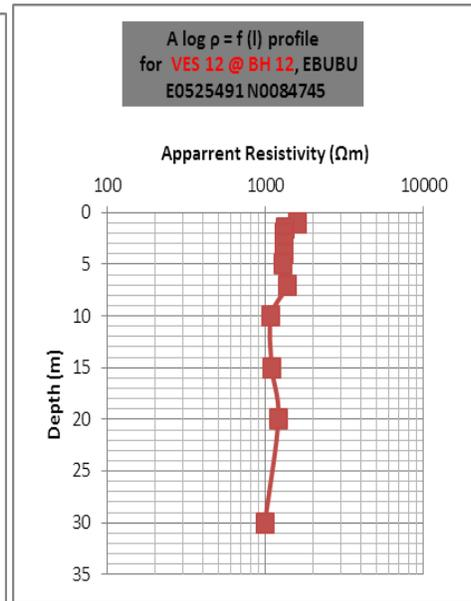
Figure 15. Resistivity log for VES 12
