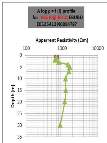
Figure 11. Resistivity log for VES 8
