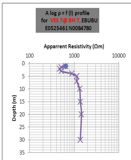
Figure 10. Resistivity log for VES 7
