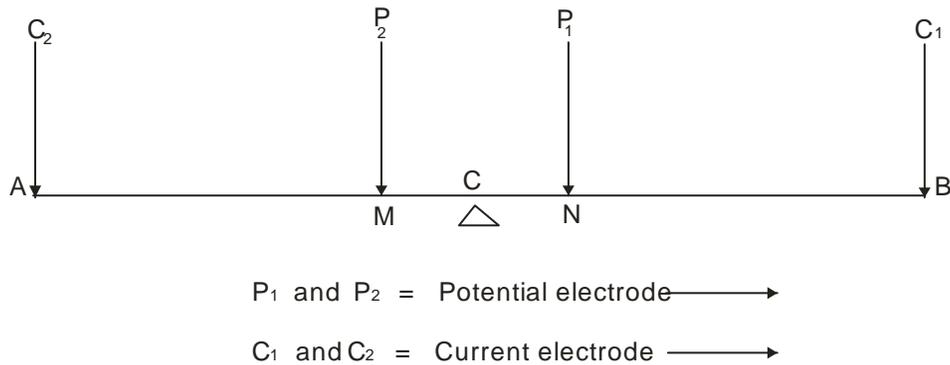
Figure 2 Electrode arrangement using Schlumberger Configuration
