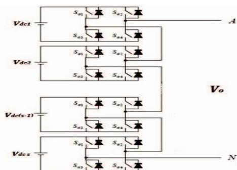
Fig.2 Cascade H-bridge multilevel inverter
