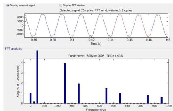
Fig.20 Source current THD under Incremental - reduction cascade H-bridge.
