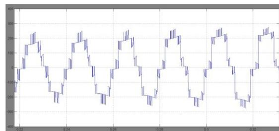
Fig.19 9-level inverter voltage under Incremental - reduction cascade H-bridge.
