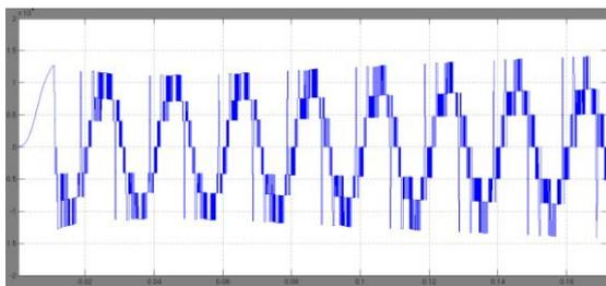
Fig.16 7-level inverters voltage under incremental cascaded I-bridge.
