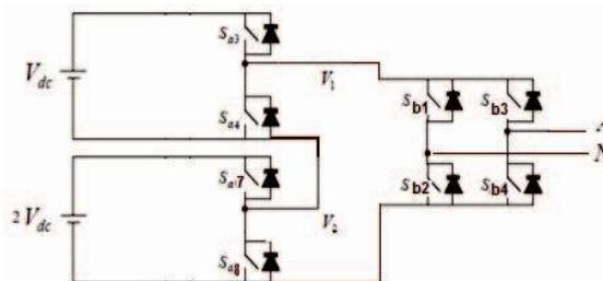
Fig.4 Incremental cascade I-bridge
