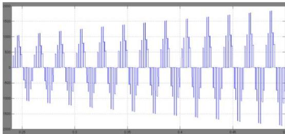
Fig.13 7-level incremental cascaded H-bridge inverter voltage
