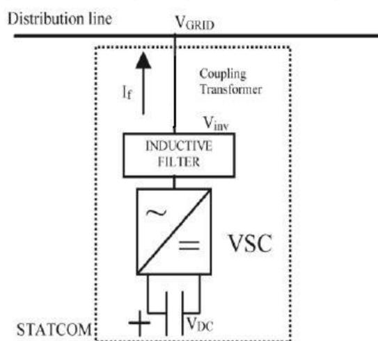
Fig.1 Basic Structure of STATCOM
