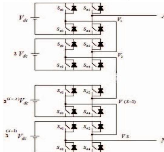
Fig.5 Incremental-reduction cascade H-bridge
