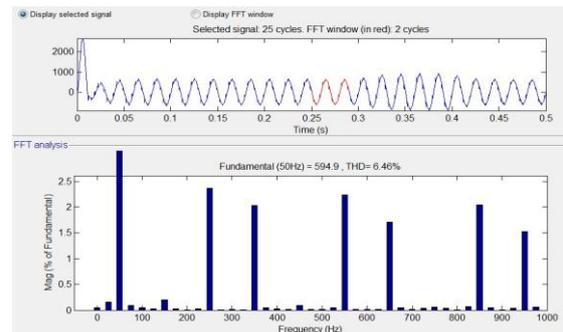
Fig.17 source current THD under incremental cascaded I-bridge.
