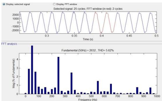
Fig.14 source current THD under incremental cascaded H-bridge.
