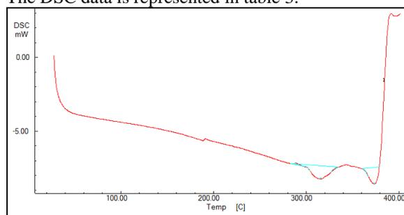
**Figure7. DSC curve of Co doped barium tartarate Crystals**
