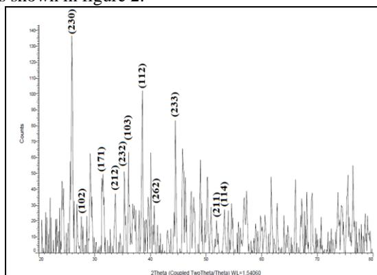
Figure2. XRD pattern of the crystals of CoBaC<sub>4</sub>H<sub>4</sub>O<sub>6</sub> 0.05M
