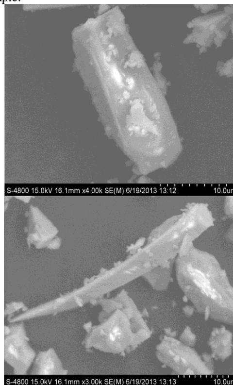
Figure 3a-b. SEM picture of 0.05M Co doped Barium tartarate crystals
