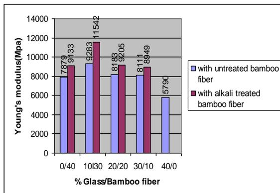
Fig.2. The variation of Flexural modulus with ratio of % Glass/Bamboo fibers reinforced polyester composites
