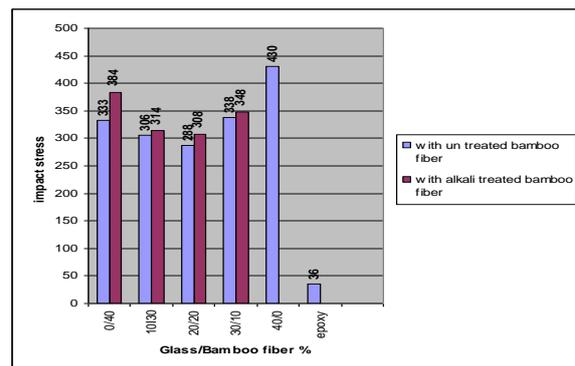
Fig. 3. The variation of impact strength with the ratio of % Glass/Bamboo fibers reinforced polyester composites
