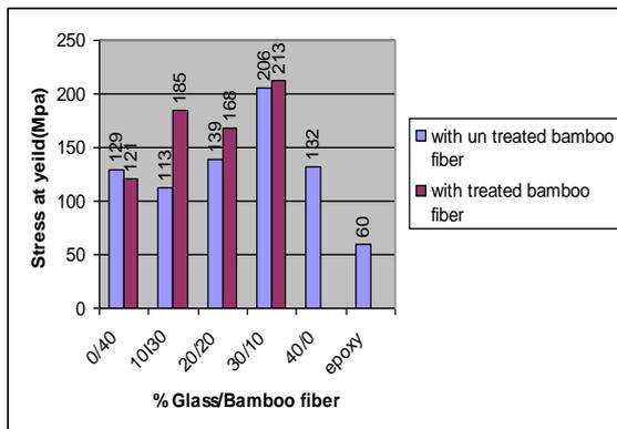
Fig.1. The variation of Stress at Yield with ratio of % Glass/Bamboo fibers Reinforced polyester composites
