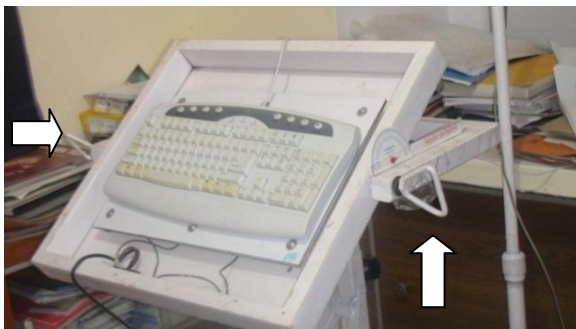
Figure 4: CNC machine panel angle adjustment mechanism
