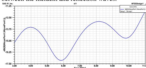
Figure 5: Return Loss parameter graph
