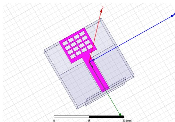
Figure 4: Geometry of the patch antenna
